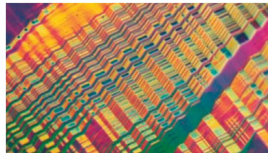
Martensite jigsaw puzzle. Bulk CuAlNi contains six different variants of orthorhombic martensite that form a jigsaw puzzle. The horizontal dimension of this image is 1.4 mm.
